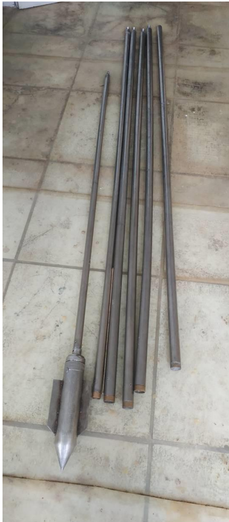
Sampling device for solids of spent ion-exchange resin and filter perlite pulp
