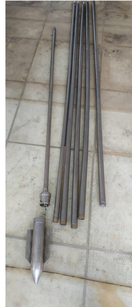
Sampling device for solids of spent ion-exchange resin and filter perlite pulp
