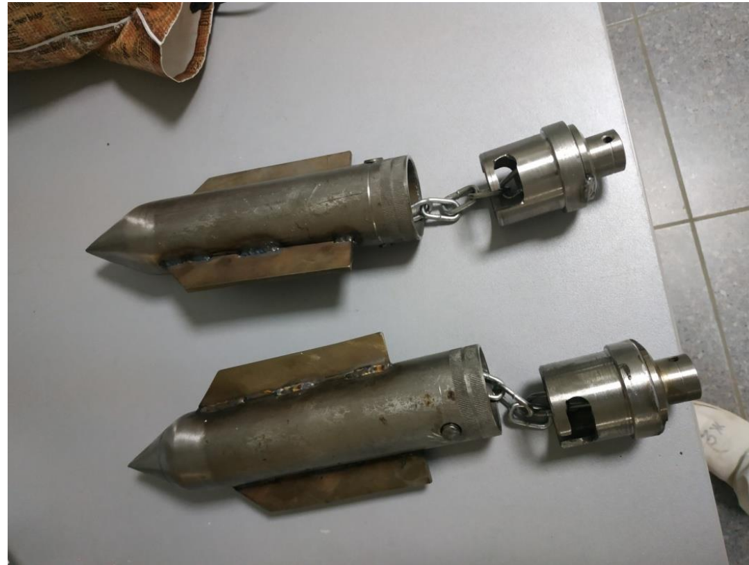
Sampling device for solids of spent ion-exchange resin and filter perlite pulp
