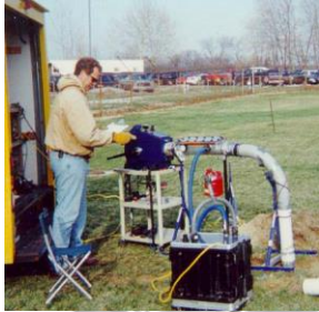
Cam & Groove cap used to insert the PNG detector into the piping system
